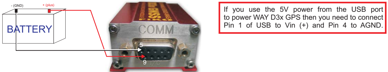
Figure 8. The pin connection for the standard version of WAY D3x GPS (outside view)
